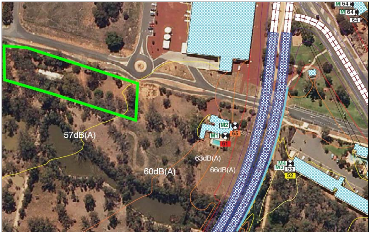
MAP 9: Noise contour map from proposed bridge with mitigation measures in place (Source: Acoustic Assessment for proposed Echuca-Moama Bridge)
